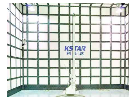
EMI laboratory (measuring RE radiation interference)
