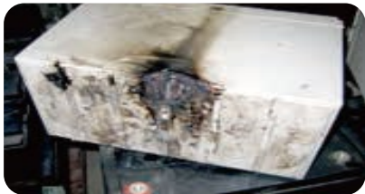
Leakage from battery bottom
